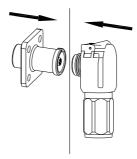
Note: Press the position indicated in the figure above before disconnecting the power terminal.
